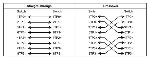
10BASE-T uses Category 3.4, 5, 5 100-ohm UTP/STP and 1000BASE-T uses Category 5 100-ohm UTP/STP for connections. Both support a maximum length of 100 meters. shows 100BASE-TX/10BASE-T pin assignments.
